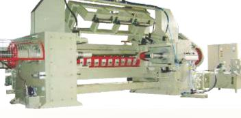
**ROTARY VENEER LATHE (4Ft SIZE) MODEL: RVT-50**
