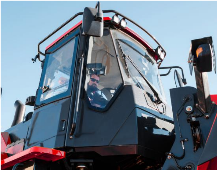
The Taylor T-1025 has been designed to offer optimized visibility. A panoramic view cab with curved front glass has been paired with well-positioned lift arms to allow the operator a clear line of sight to the attachment at ground level.
