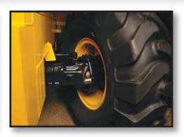
**AXLES:** Planetary gear reduction at each hub allows efficient power transfer to the ground while 20 degrees of total axle oscillation maintains traction at all times.
