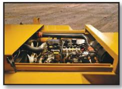
**ENGINE:** Powerful Perkins 4-Cylinder Tier 3 (Stage IIIA) Turbo Diesel offers minimal fuel consumption with simplicity of maintenance through easy access sliding hood. Optional 6-cylinder Turbo Diesel available.
