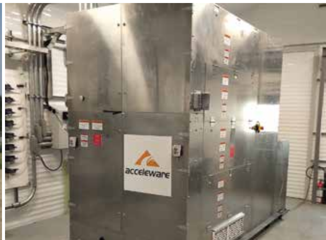
Acceleware's 2 MW Clean Tech Inverter (CTI). The CTI converts electricity to radio frequency energy, allowing for the electrification of industrial heating. PHOTO COURTESY IMII AND ACCELEWARE.
