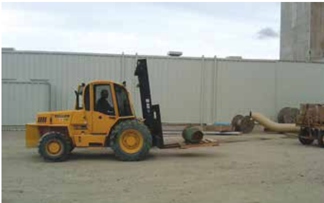
S120 4x4, 12,000 lbs. capacity, full ROPS Cab, Surface.
