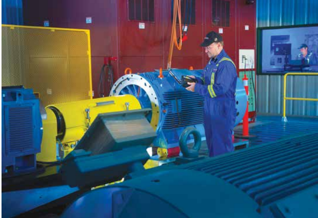
WEG miner head motor set up for a loaded test on PEM's regenerative dynamometer.
