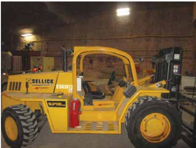
SLP-100 4x4, 10,000 lbs. capacity low profile (75-inch) ROPS canopy.
