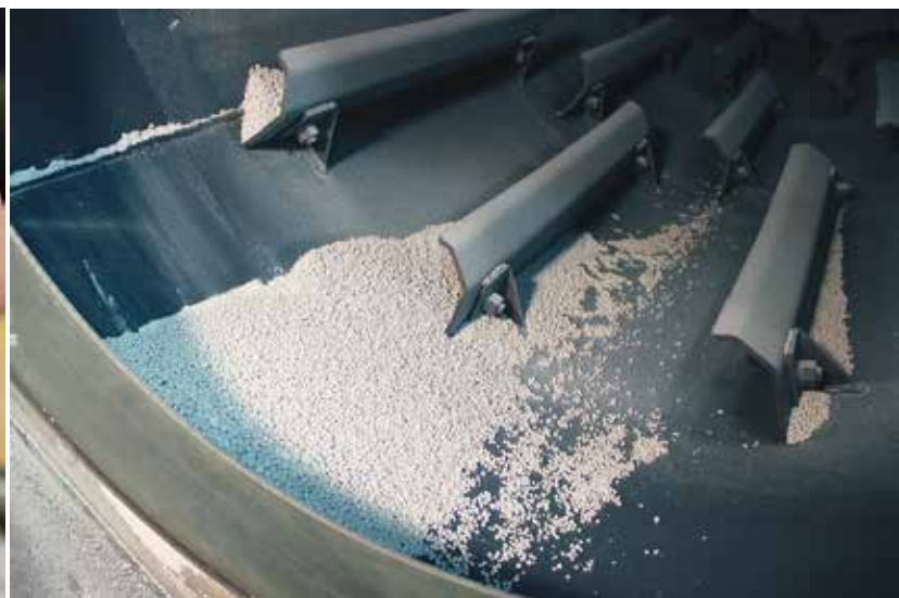
Potash granules in the Innovation Center's pilot rotary dryer.
