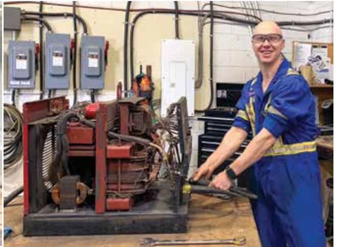
Kurtis Dyck, welder service foreman, finishes up testing a repaired Lincoln Electric Idealarc CV-305 MIG welder.
