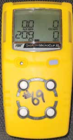
Electronic portable gas detectors are handheld units that are often programmable, and they provide instantaneous measurements to the operator of the equipment.
