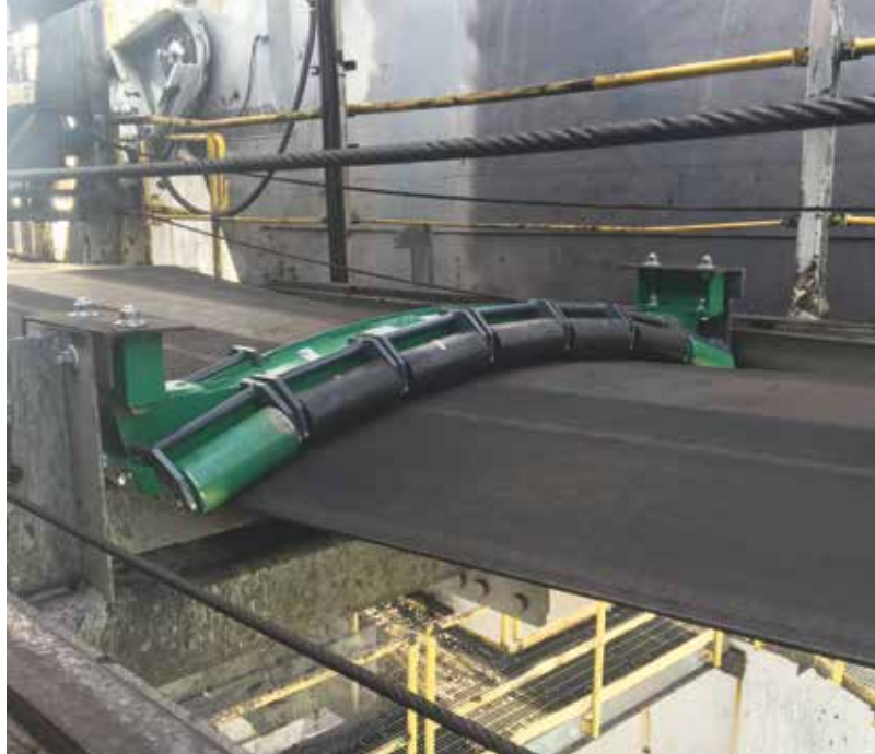
ON-Track® Belt Tracking Idler application.
