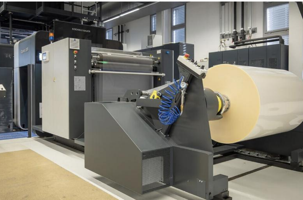
RS 106 X reel-to-sheet feeder in production with IML film
