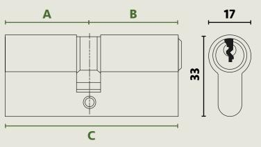
To determine size of cylinder, measure 'A' then 'B' Example A = 40mm, B = 45mm order 40/45 cylinder
