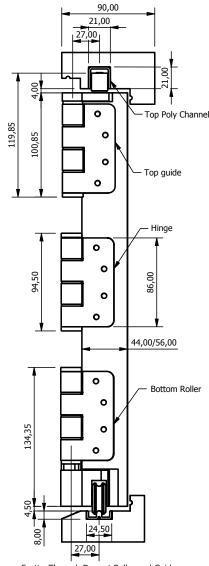
SectionThrough Door at Roller and Guide
