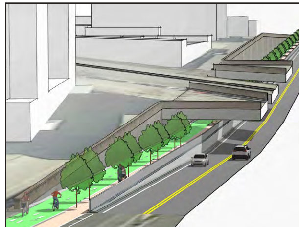
Viaduct - proposed condition separates cyclists and pedestrians with elevated path on one side.
