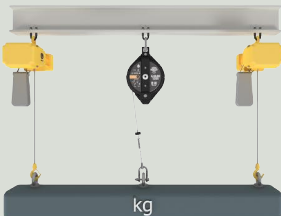
Multiple Hoist Installation
