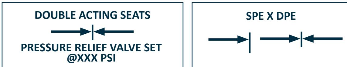
Valves with two double isolation seats will be supplied with a pressure relief valve in the upper end of body, unless specified otherwise during order. This valve relieves pressure in cases of thermal pressure buildup in the closed position. See Body Pressure Relief section for pressure relief settings on the valve.
