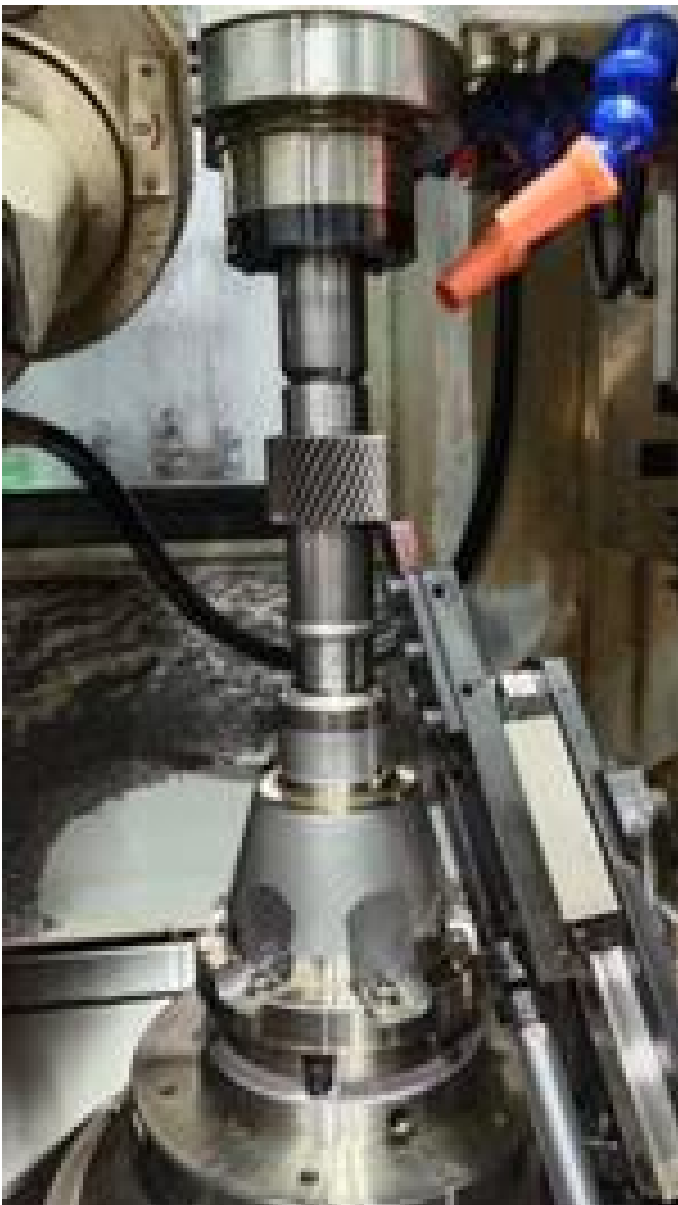
The segmented clamping bushing of the Mando G211 mandrel is vulcanized and thus dampens vibrations during machining. The service life of the tools has increased since using the mandrel.
