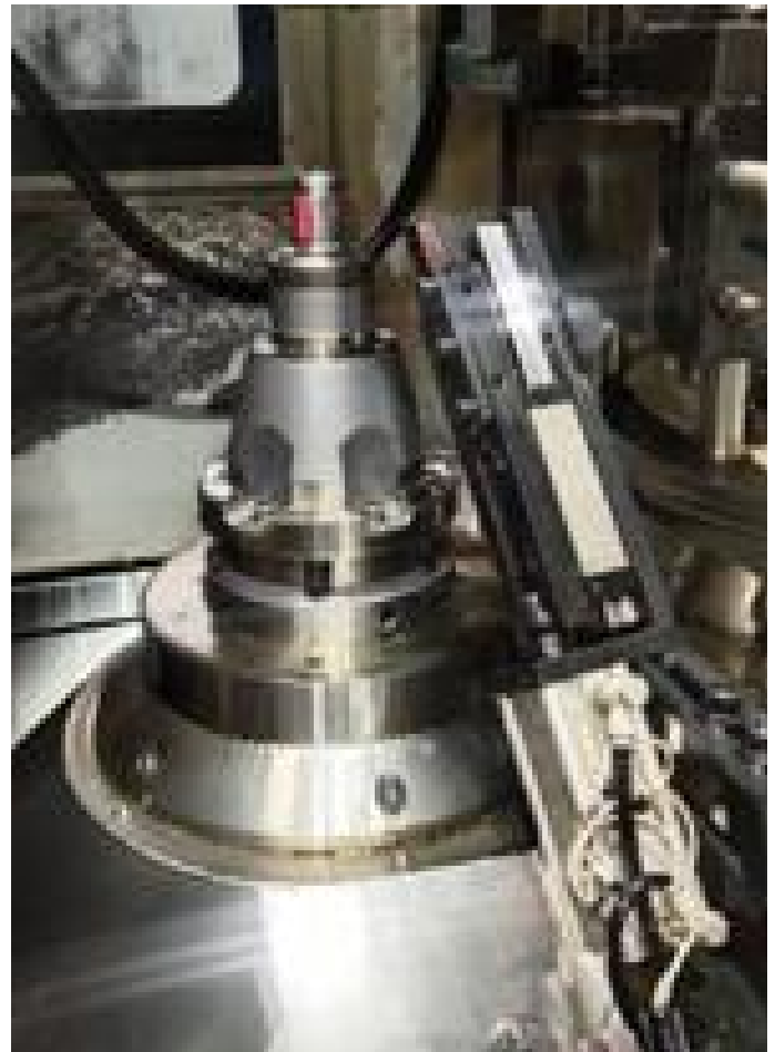
The Mando G211 mandrel clamps radially with a pull-back effect. Depending on the mandrel size, the radial clamping force of the mandrel is 42 - 150 kN.
