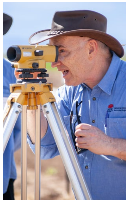
NRAR staff using a dumpy level to measure dam size. Photo: NRAR
