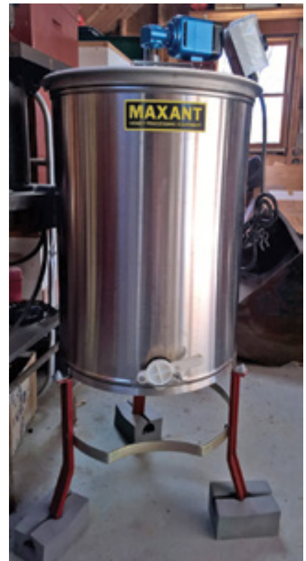
Canoe pads being used to restrict extractor vibration.
