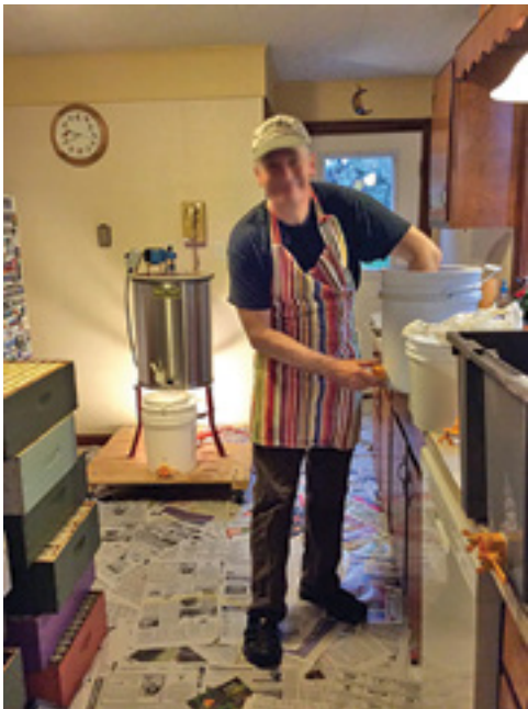
A wheeled extractor platform. Much of the vibration is absorbed.
