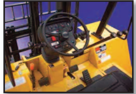
STEER COLUMN: Self contained, fully adjustable, tilt and telescopic steer column.
