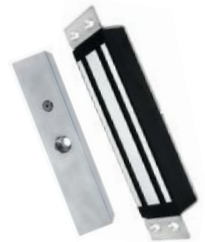
Aluminium-zinc, mortise-mount, fail-safe, 270kg holding force, 12V/24VDC
