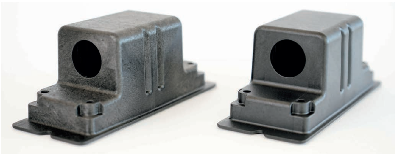
Two injection-molded sensor housings from Sick: With surface defects (streaks, left) and after optimization of machine settings (right).
