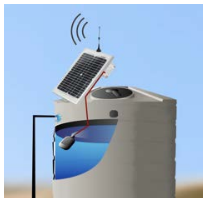
Transmitter at Tank End
