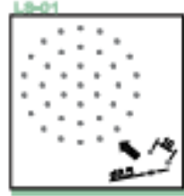
L0-01 Hole size : 0.5x0.5mm Pitch : 1.5mm Open Area : 5.4%
