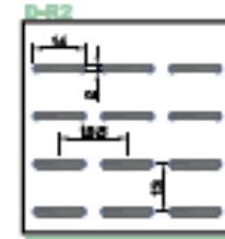
D-02 Hole size : 0.5x2.0mm Pitch : 1.5mm Open Area : 11.25%
