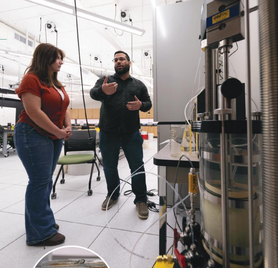
From left, Ashley Rimmel learns from assistant professor Iuri Santos about how to use a triaxial machine in SRU's lab that tests properties of soil.
