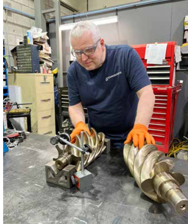
A Comairco technician inspects a clean rotor (far) and a varnished rotor (near).
