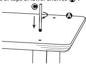
Shelves **A** are securely stacked by placing Legs **3** over Stabilizer Pins **6** and pressing down until flush.
