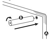
Stabilizer Pins are screwed into at least two corners of tops of lower Shelves .
