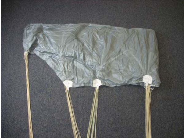
Grasp the B-line group under slight tension and fold over the A-line group.
