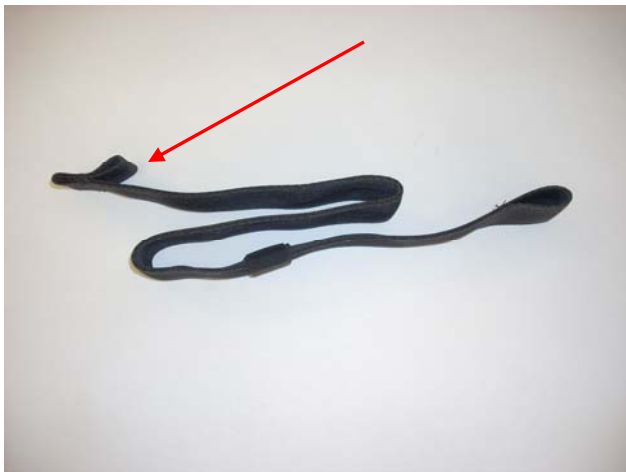
Pictured above is the other half of the Belly-Band. When installing it to the Left Side of the TPDS MSS be sure that the "turned back" end is facing the Harness/ Container to prevent it from slipping when fed through the Friction Adapter.
