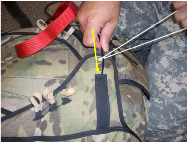
Insert one of the plastic covered cables through the closing loop then into the channel as shown.
