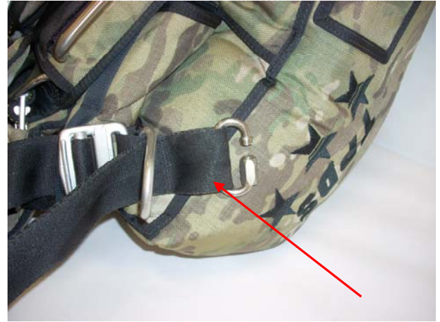
Pass the strap through the slot of the RW-8 Harness Ring of the lower Left Side of the TPDS MSS .
