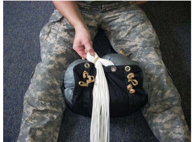
Stow the first bight of line into a rubber band brought through one of the center grommets.
