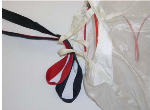
Pass both loops through both loops of the Spring-loaded Pilot Chute.
