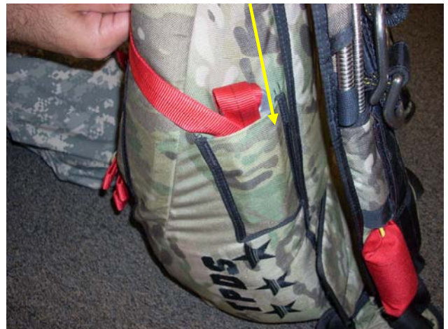
Stow the remainder of the Static Line and the Static-line Snap into the pocket on the side of the Container.
