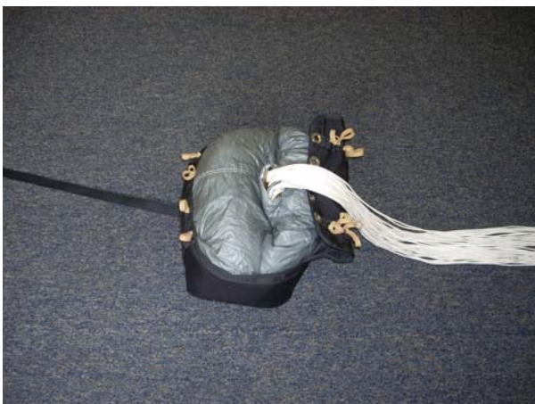
Bring the lines up through the center of the canopy and out of the Deployment Bag.
