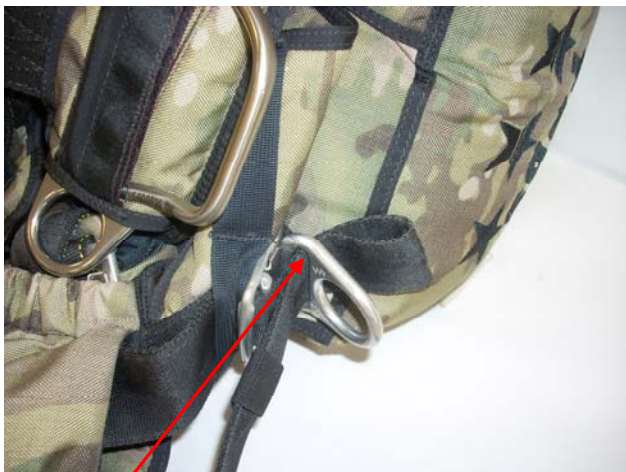
Pictured above is the other half of the Belly-Band. When installing it to the Left Side of the TPDS MSS be sure that the "turned back" end is facing the Harness/ Container to prevent it from slipping when fed through the Friction Adapter.
