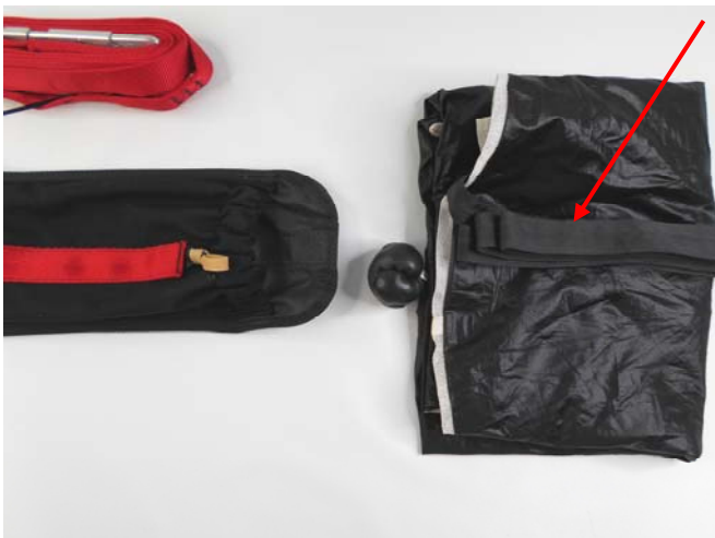
"S"-Fold the bridle in the middle of the P/C.
