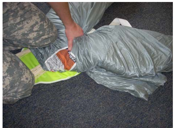
Place free-bag under the reserve with the trailing edge in line with the mouth of the bag.
