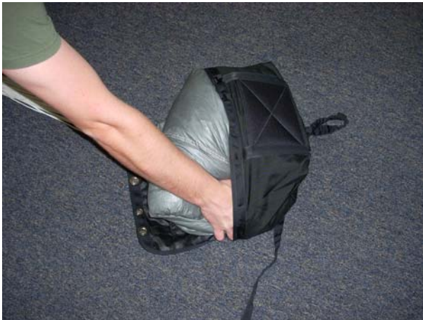
Insert the other corner of the canopy into the other corner of the Deployment Bag.
