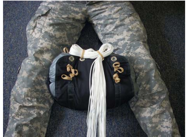
Stow the second bight through a rubber band brought through the other center grommet.
