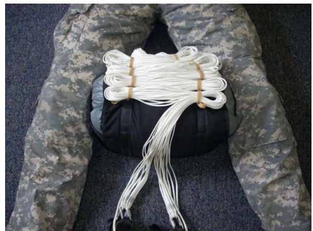
Continue stowing the lines, alternating back and forth, until approximately 12"-16" remain.
