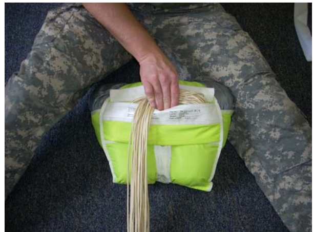
Take the second line bight and place it into the opposite corner of the line pouch.
