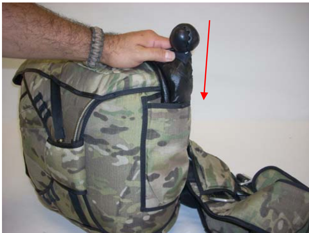
Place the Pilot Chute into the Pouch on the Bottom of the Container.
