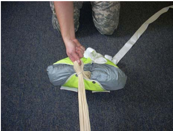
Close the free-bag by feeding the safety stow through the grommets of the free-bag and make the first line bight approximately 1 1/2” and place in the safety stow.
