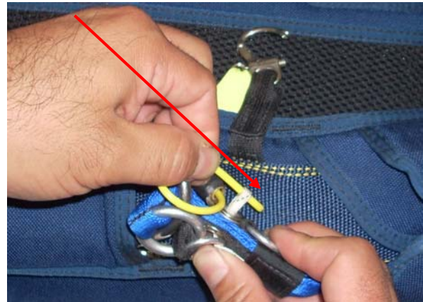
From the back side of the Riser, feed the loop through the housing grommet.
