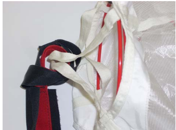
Pass the ends through both of the loops at the same time, forming a double loop. Tighten the formed knot.
