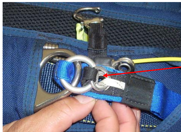
Pass the Type IIA loop through the small Riser ring and into the grommet.
