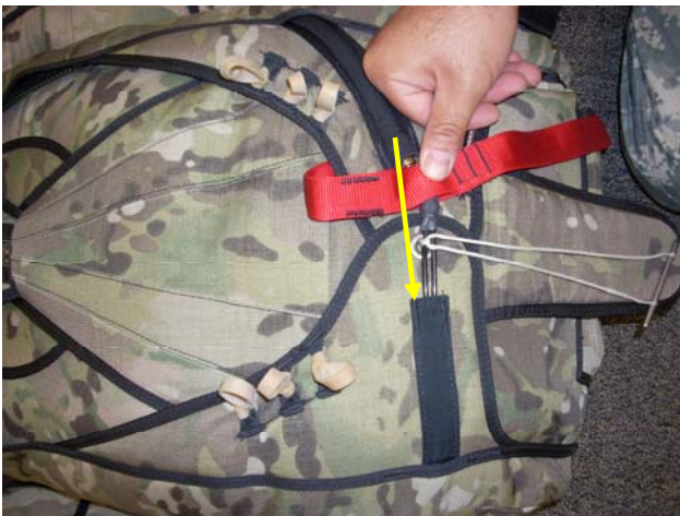
Insert the other plastic covered cable into the channel.
