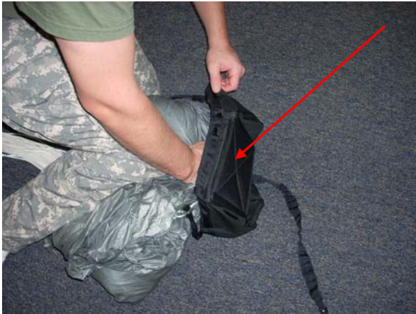
With the Kicker Plate facing up place one corner of the canopy stack into the Deployment Bag.
