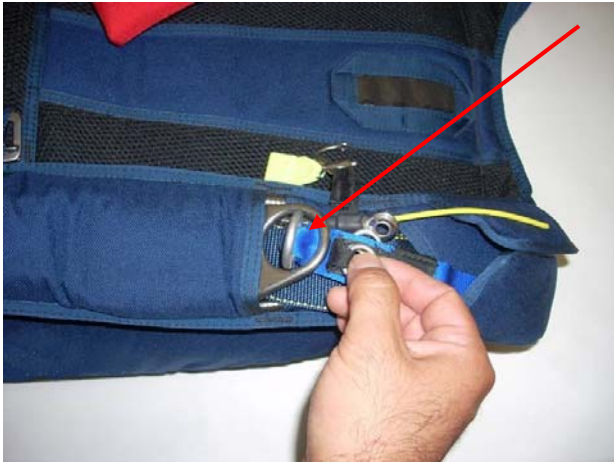
Pass the large ring of the Riser through the large ring of the Harness .
