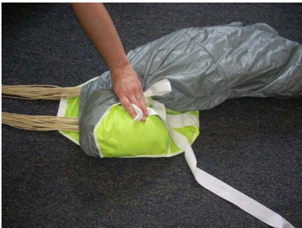
Put all of the fabric from one ear into the free-bag, filling out the ear of the free-bag. Repeat for the opposite ear; wrap free-bag around the “S”-folded portion of the parachute.
