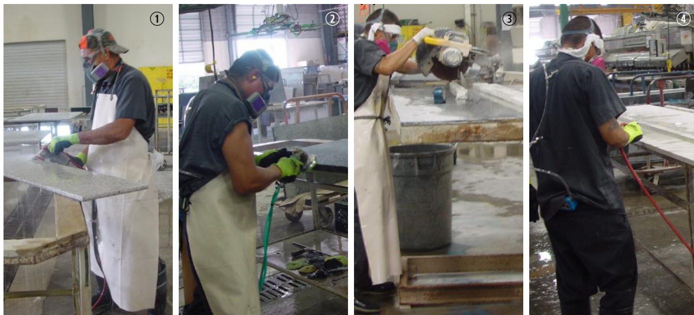
1. A worker using a handheld pneumatic wet grinder with a diamond grinding cup wheel in the final grinding process; 2. A worker using a handheld pneumatic wet polisher in the polishing process; 3. A worker using a wet miter saw in the lamination process; 4. A worker using compressed air to dry the surface of the stone in the lamination process. Images courtesy of the National Institute for Occupational Safety and Health.
