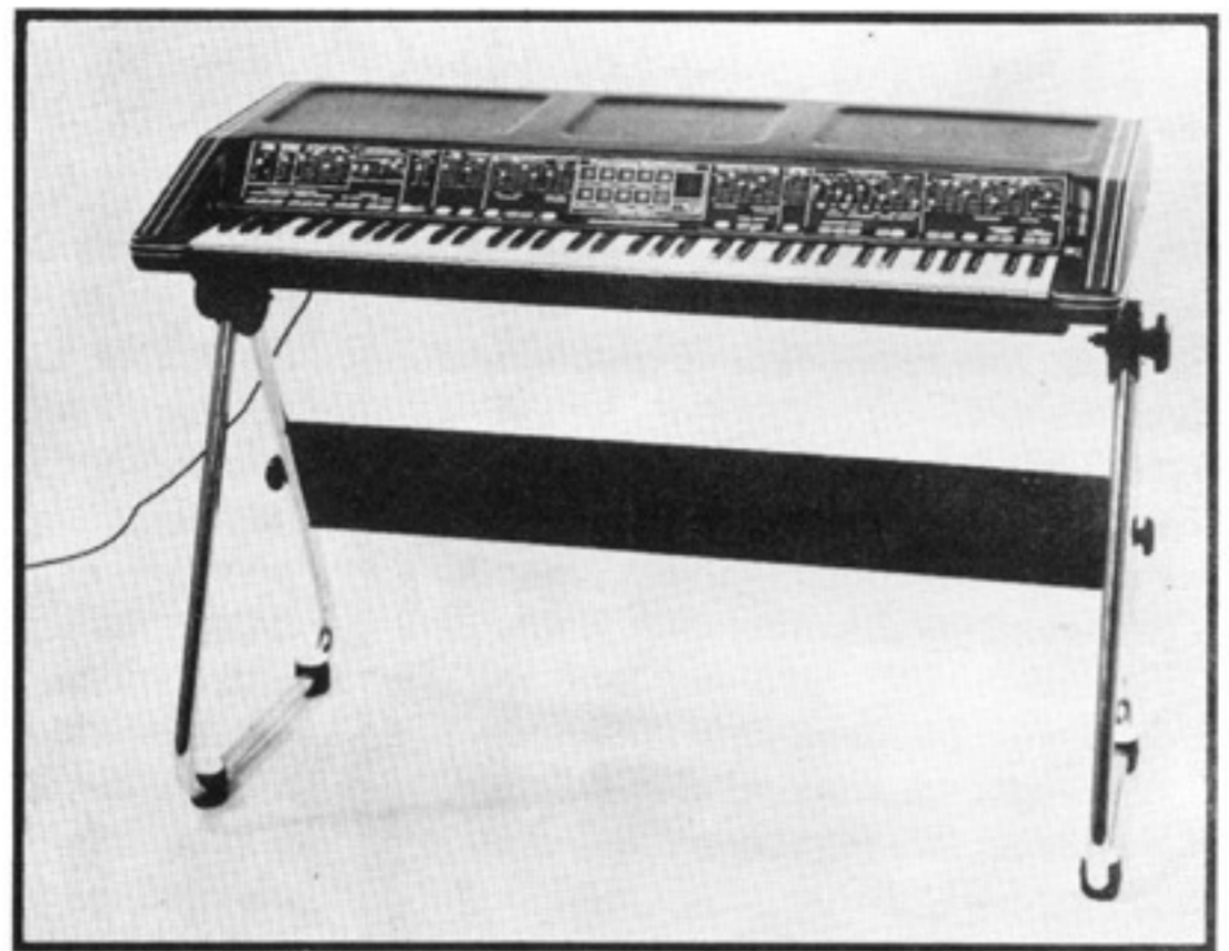
The Polymoog's keyboard is touch sensitive and reaches nearly six octaves. Moog spent $100,000 developing a single IC that would perform the functions of two envelope generators, a VCA and a VC filter.
