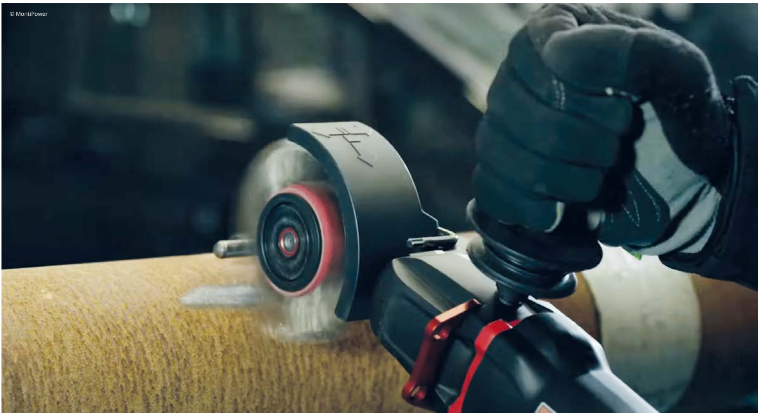
The MontiPower® technology is designed to visibly clean and create roughness profiles without any loose abrasives and without the creation of paint or rust dust.
