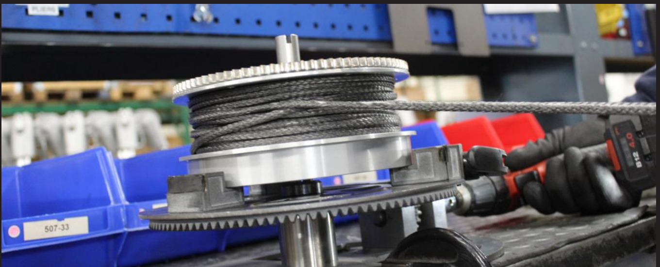
High grade synthetic rope being fitted to a SAVER rope drum
