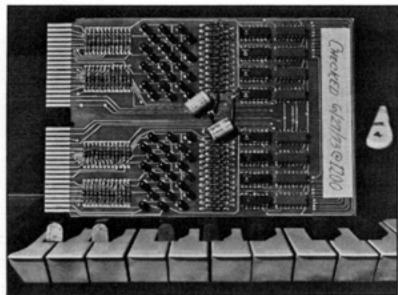
A key circuit from Knowlton's interface system.
