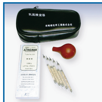
AS-1 Air Flow Indicator determines the velocity and direction of air flow.
