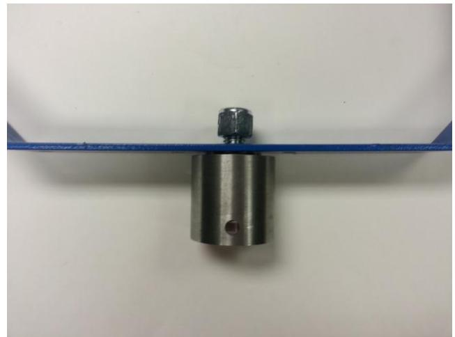
4. Attach Oscillator Linkage Bolt to Oscillator Arm. Tighten Nut on to bolt as far down as possible.
