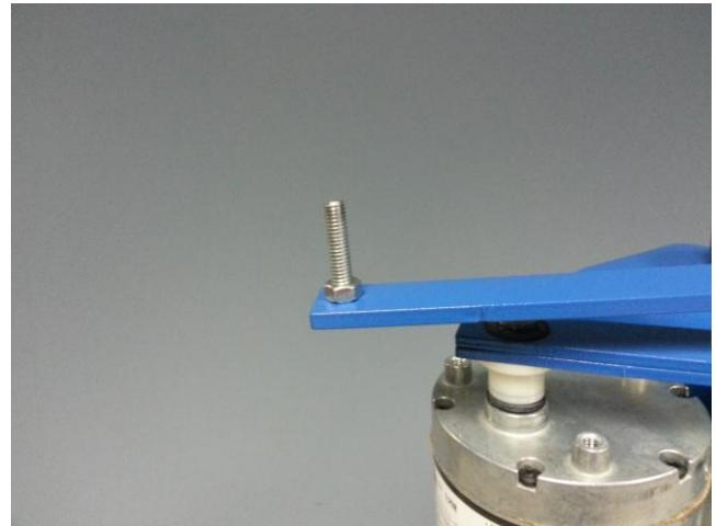
5. Place white larger spacers onto bolt from previous step. Save the smaller **BLUE** spacer and nut for later.
