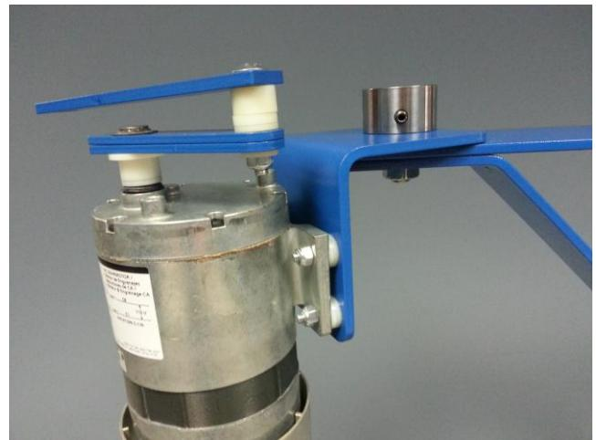
3. Attach the Yoke Bearing Assembly to the bottom of the supplied yoke. **Toque Nut to 100 foot pounds.**
