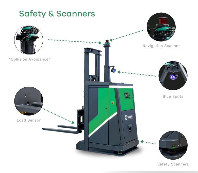
The AGVs are equipped with advanced safety systems designed to protect employees, infrastructure, and the robots themselves.
