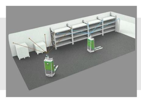
The Counterbalance utilizes natural navigation with top-mounted laser scanning to ensure precise and reliable movement.
