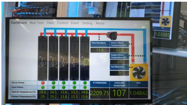
Figure 6 – SJI Real Time Display of pPUE 1.04 for Data Servers Operation
