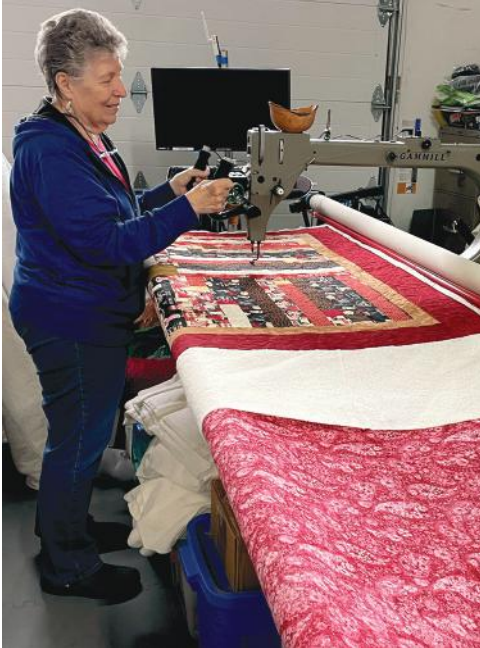
Jane Adams operates the long arm quilting machine. While many quilters still stitch by hand, the long arm quilter simplifies the process. The stitching pattern adds an important design element to the finished piece.
