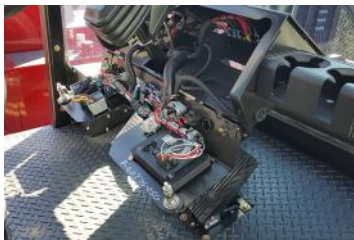
Flip-down Dash with Color/Number Coded Wiring (Standard)
