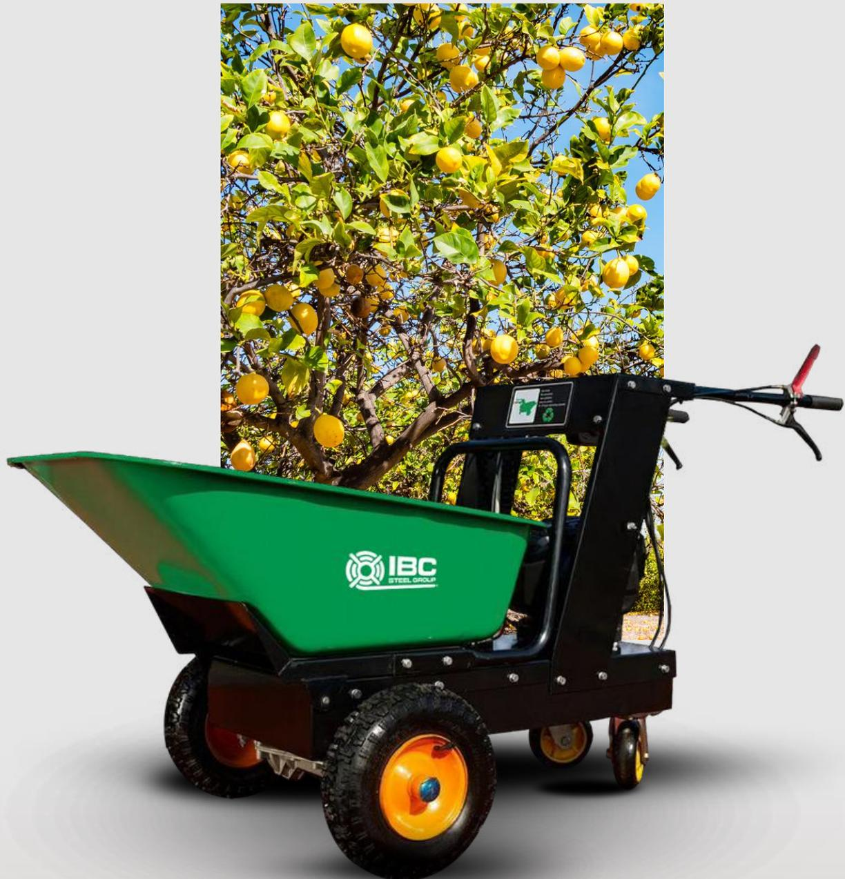
**Battery:** Lead-acid (48V, 4\*20Ah)
