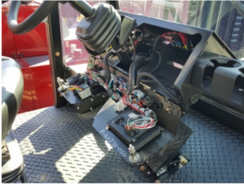
Flip-down Dash with Color/Number Coded Wiring (Standard)
