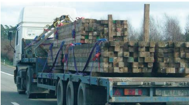
The load above is well lashed for transport. The individual timber packs are lashed together and then the entire load is lashed to the truck. Dunnage is also used to limit movement of the load during transport.
