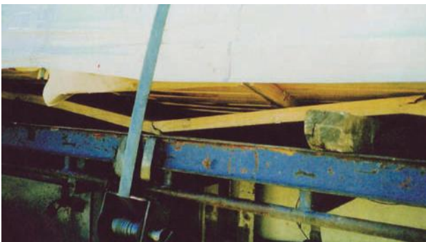
The base of the load broke from the webbing tie-down force. The webbing tie-down should have been positioned above the dunnage supporting the load.
