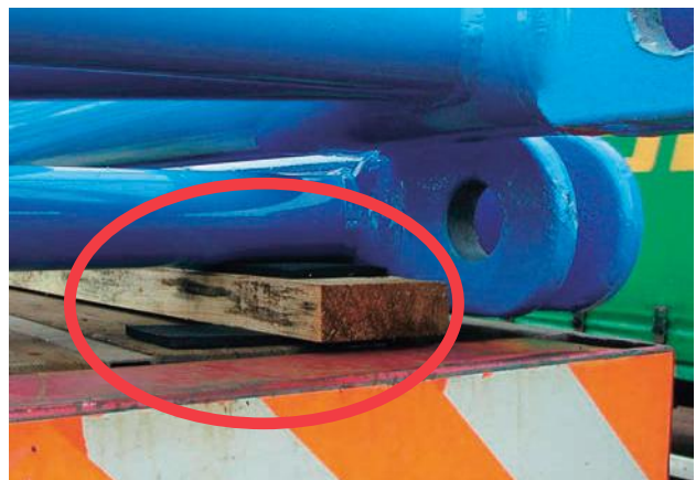
Anti-slip mat used with dunnage is an effective means of stabilising the load and reduces the likelihood of the load moving during transport.
