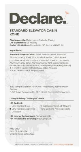
FIGURE 5-18 Declare Label for Kone Standard Elevator Cabin
