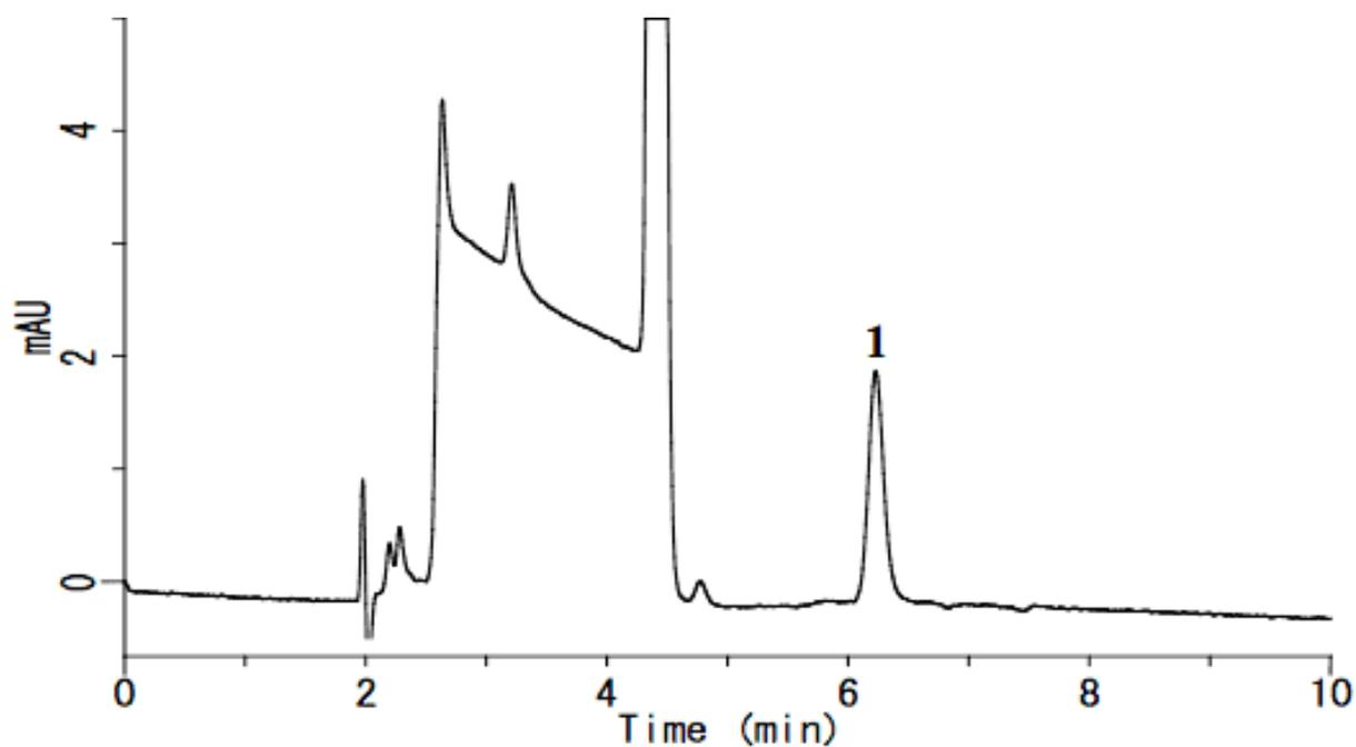
System : GL-7400 system Solutes : 1. Ascorbic acid(Deriv)(1 mg/L)
