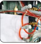
3\* regulators for controlling the water flow of cup filling. Spittoon rinsing and air flow of air suction
