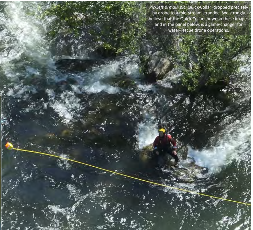
The drone flies 30-50ft past the rescuer drop point to counter the snap back recoil upon release. The harder the pull on the drone, the greater the recoil.
