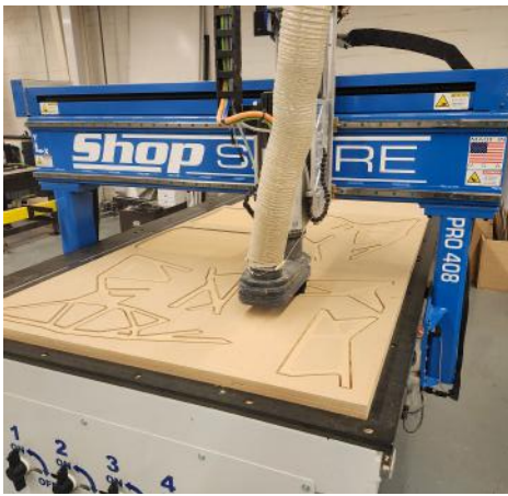
Fabrication Stage I: 3-axis milling of chair parts.
