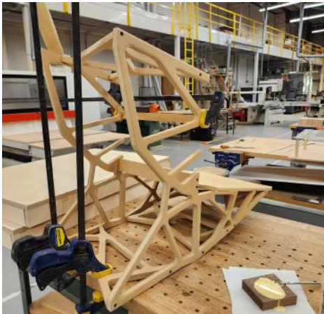
Fabrication Stage III: Assembling and screwing the chair components together to enhance structural stability.
