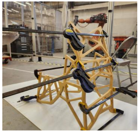
Fabrication Stage II: Gluing the structural parts.
