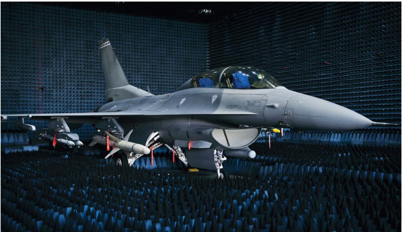
Aircraft on test in anechoic test chamber*
