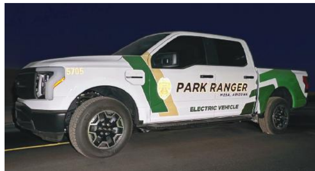
This Mesa, AZ park ranger vehicle is a partial wrap featuring V4000 Reflective Film and PVC-Free DOL 6460 Gloss and MPI 1105. Photo courtesy of VisionIT Media
