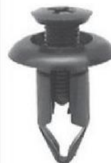
21123 (75867-30120) Black Nylon Rocker Moulding Push-Type Retainer Head Diameter: 18mm Stem Length: 19mm Fits into 8mm Hole Lexus GS350, GS430, GS460 & LS460 and Toyota Camry 2007 - On
