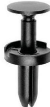
20966 (5160260-AA) Black Nylon Rear Bumper, Tail Light & Fender Push-Type Retainer Bottom Head Diameter: 18mm Stem Length: 20mm Fits into 8mm Hole Dodge Caliber and Jeep Compass & Patriot 2007 - On
