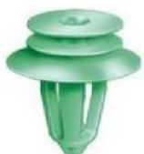
20879 (007-988-99-78, 007-988-34-78) Green Nylon Door Trim Panel Retainer Overall Length: 19.5mm Mercedes-Benz 1996 - On
