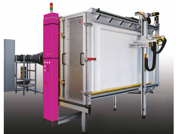
Photo : Essai de scanning - EN1822-4
