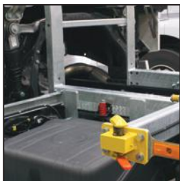
Galvanised steel sub frame with steel front bulkhead up-stand
