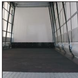
21mm phenolic plywood floor
