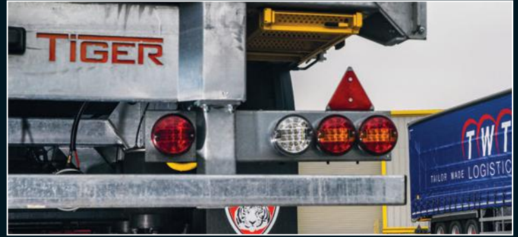
Galvanised rear under-run bar
