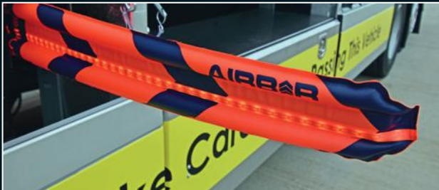
NuVech Solutions 'AirBar' self-inflating LED safety barrier
