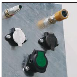
Galvanised front nose box with heavy duty lead-up
