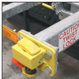
Retracting location dishes and ISO twist locks to suit new/existing equipment
