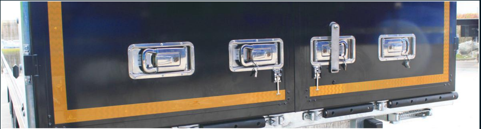
Flush doors with recessed lock handles
