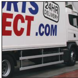
Aluminium alloy bearers and side rave with concealed fastenings
