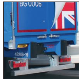
Hot-dip galvanised bolt-on under-run bar
