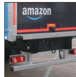
Hot-dipped galvanised under-run bar
