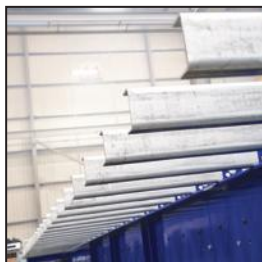
Galvanised floor bearers and V-groove side rave
