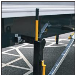
Handle-operated, pull-out, drop-down, braced telescopic support legs [optional]
