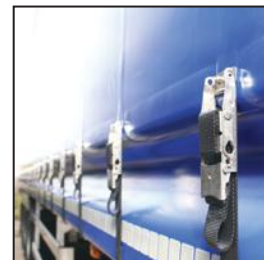
Stainless steel, bolt-on locking buckle
