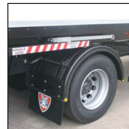
Thermoplastic mudwings with spray suppression
