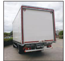
Hot-dipped galvanised rear frame with integral drain channel
