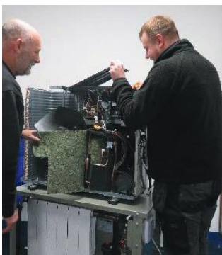
A mobile air source heat pump unit used in training at Gastec, Milton Keynes Photo credit: Gastec
