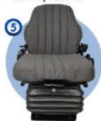
Dust cover fitted and seat fully restored.
