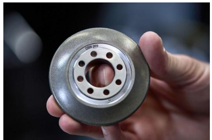
Picture 4: With CBN pro, the new tools from KAPP NILES, surface qualities of Ra < 0.2 \mu m can be achieved on the workpiece.
