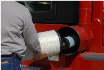
Donaldson Air Cleaner with Safety Element (Standard)
