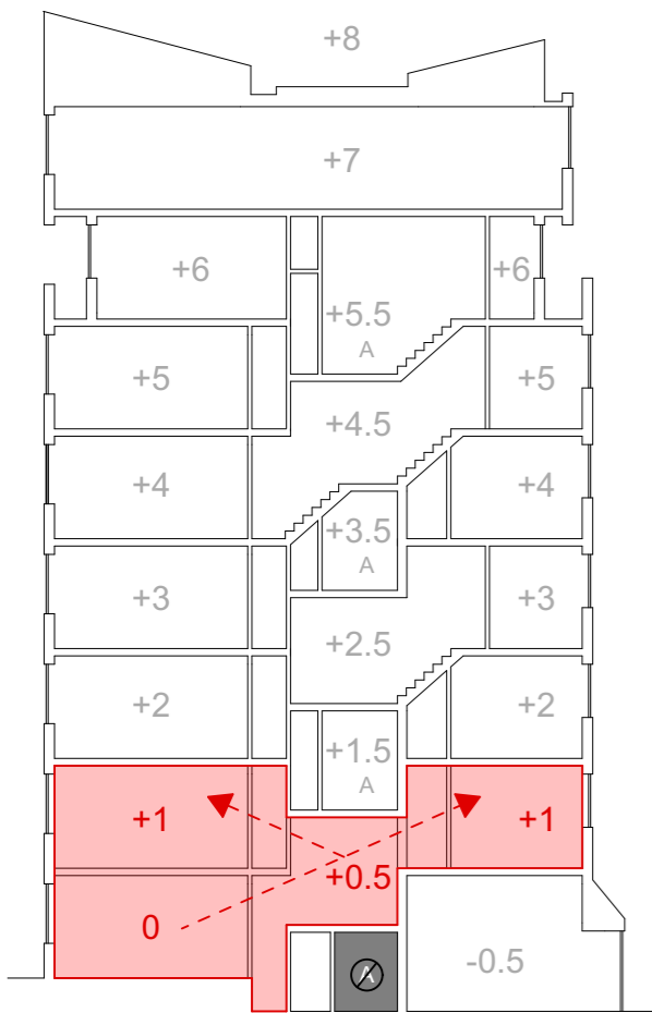
CROSS SECTION_1:200 A = Access Corridor
