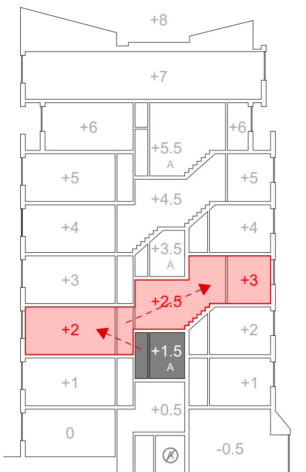
CROSS SECTION_1:200 A = Access Corridor
