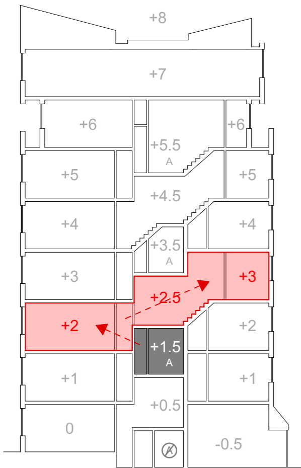
CROSS SECTION_1:200 A = Access Corridor
